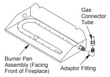
Figure 9 - Installing Burner
